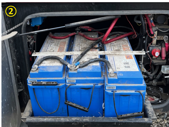
600 amp hours of lithium batteries fit in the same space as six 6v batteries.
